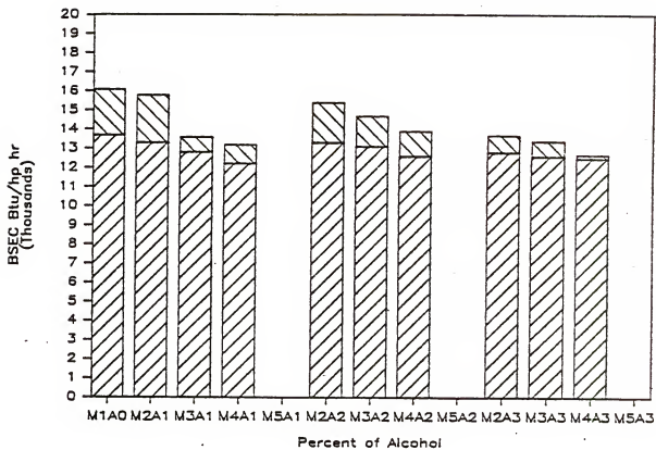
FIG. 5-21 UNCERTAINTY IN BSEC VALUES AT PHI1, S3, AND 2500 RPM.
