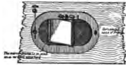
Mode of mounting the semi-transparent mirror N so as to give altitude and azimuth movements to the reflected beam
