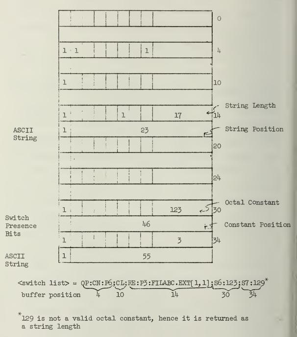
Figure IV.3 The Buffer Returned on Parsing a Switch List
