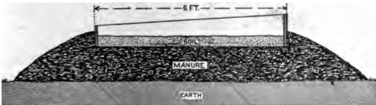
FIG. 6.—Cross section of a temporary hotbed.
