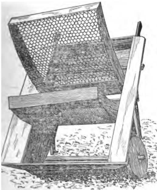
FIG. 7.—Details of the construction of the first berry harvester.
