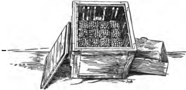
FIG. 11.—Refrigerator shipping case.
