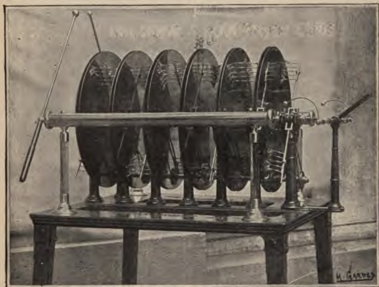
FIG. 25.—EBONITE PLATE WIMSHURST MACHINE.
