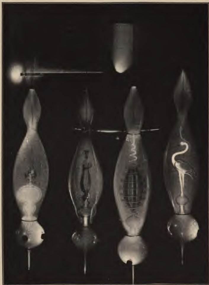
FIG. 33.—PHOTOGRAPH SHOWING THE EFFLUVE FROM THE TOP OF THE RESONATOR, AND GEISSLER TUBES LIT UP BY INDUCTION.
