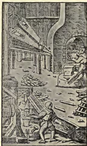
FIG. 3.—A blast furnace of the Middle Ages
