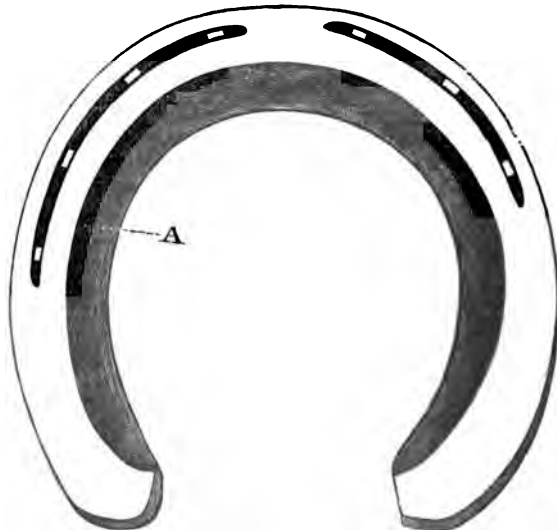
FIG. 3.—HUNTING SHOE FOR OFF FORE FOOT, CONCAVE ON THE GROUNDED SIDE.
