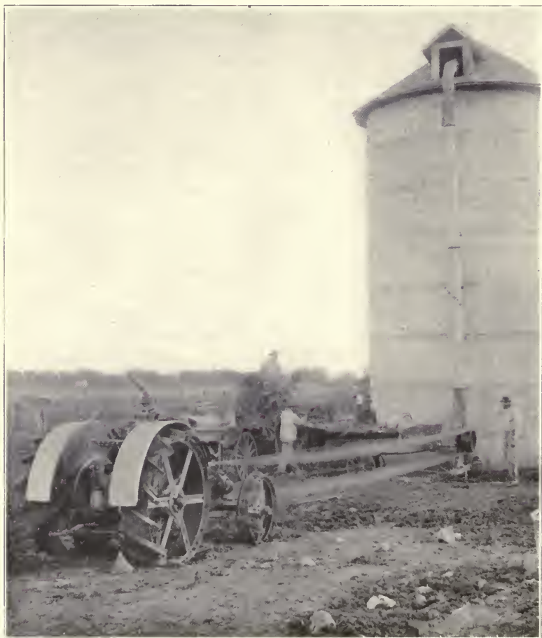
FIG. 20.—A WIDELY USED THREE-PLCW MODEL Silage cutting is one of the most important belt-power jobs.
