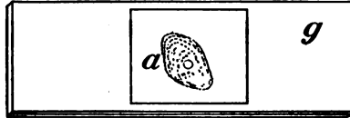
FIG. 172. — Spot a , on a glass slide g , touched with the thumb moistened from the lips as in turning the pages of a book.
