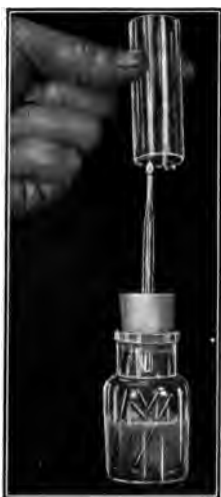
FIG. 17.— Making hydrogen. The bottle contains five nails and weak sulphuric acid. To the right of the flame of hydrogen at the tip of the glass tube are two drops of water formed by the union of the hydrogen coming out of the bottle and the oxygen in the air.
