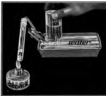
FIG. 18.— Making oxygen. e , rubber tube; n , chlorate of potash and black oxide of manganese; o , oxygen which is bubbling out from t , the test tube.
