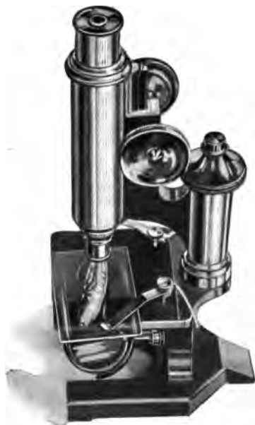
FIG. 82.— Microscope arranged to see the blood circulating in the tail of a tadpole.
