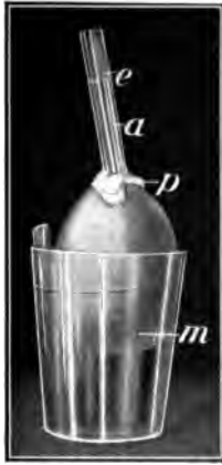
FIG. 66. — Egg experiment, showing osmosis. The shell is removed from the egg at m so as not to break the membrane lying close within it. a , glass tube; p , paraffin; e , height to which the contents of the egg were forced in an hour.
