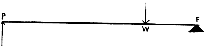
FIG. 37.—A lever of the second order. F , fulcrum; P , power; W , weight. The arrows indicate the direction in which the forces act.
