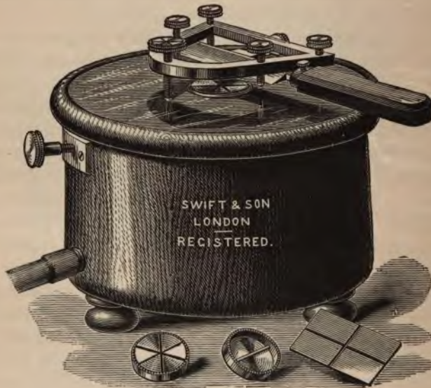
FIG. 11.—WILLIAMS' FREEZING MICROTOME.
