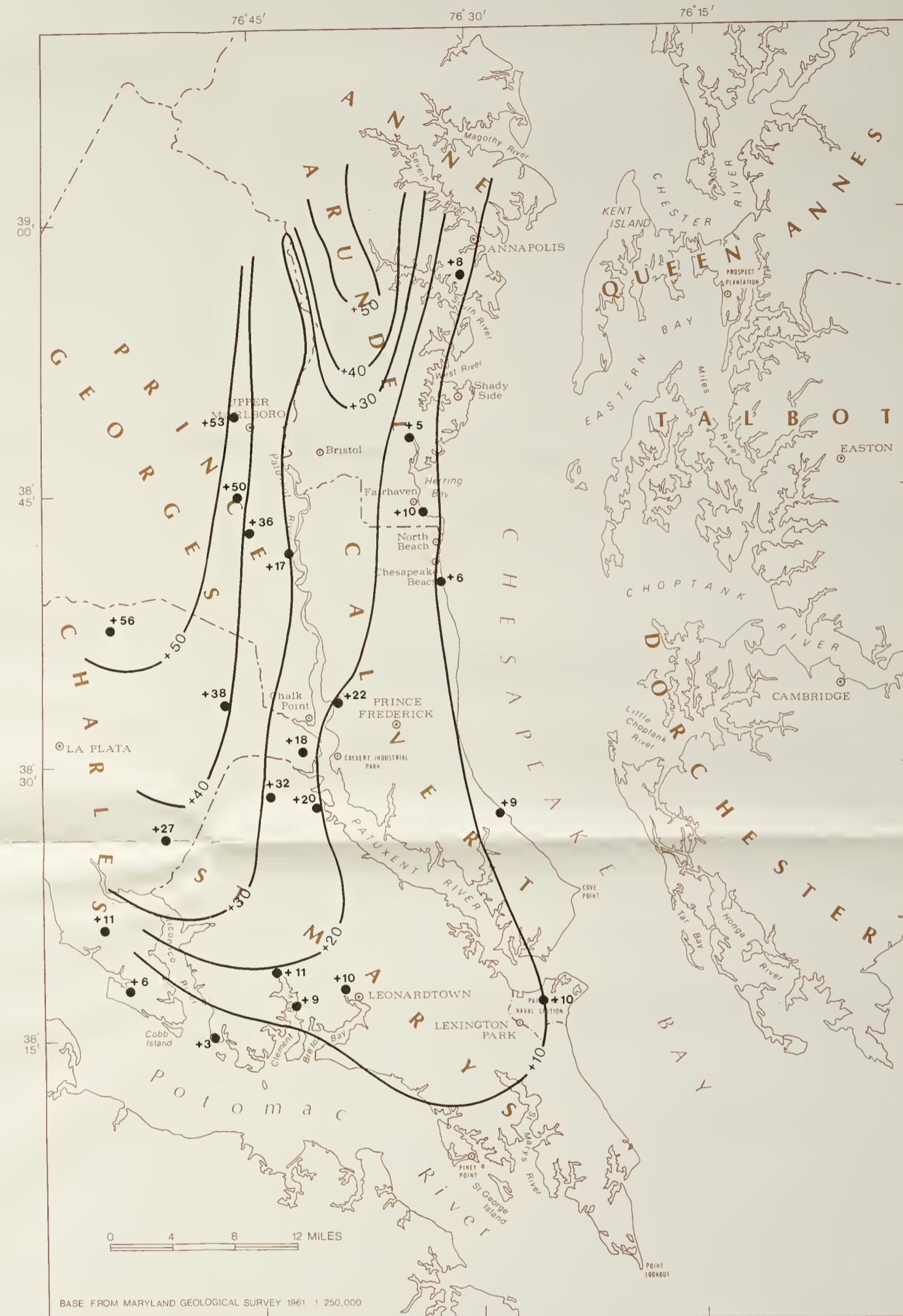
Simulated pre-pumping potentiometric surface and water levels measured early in aquifer development as reported by Darton (1896), Clark and others (1918), and Otton (1955).
