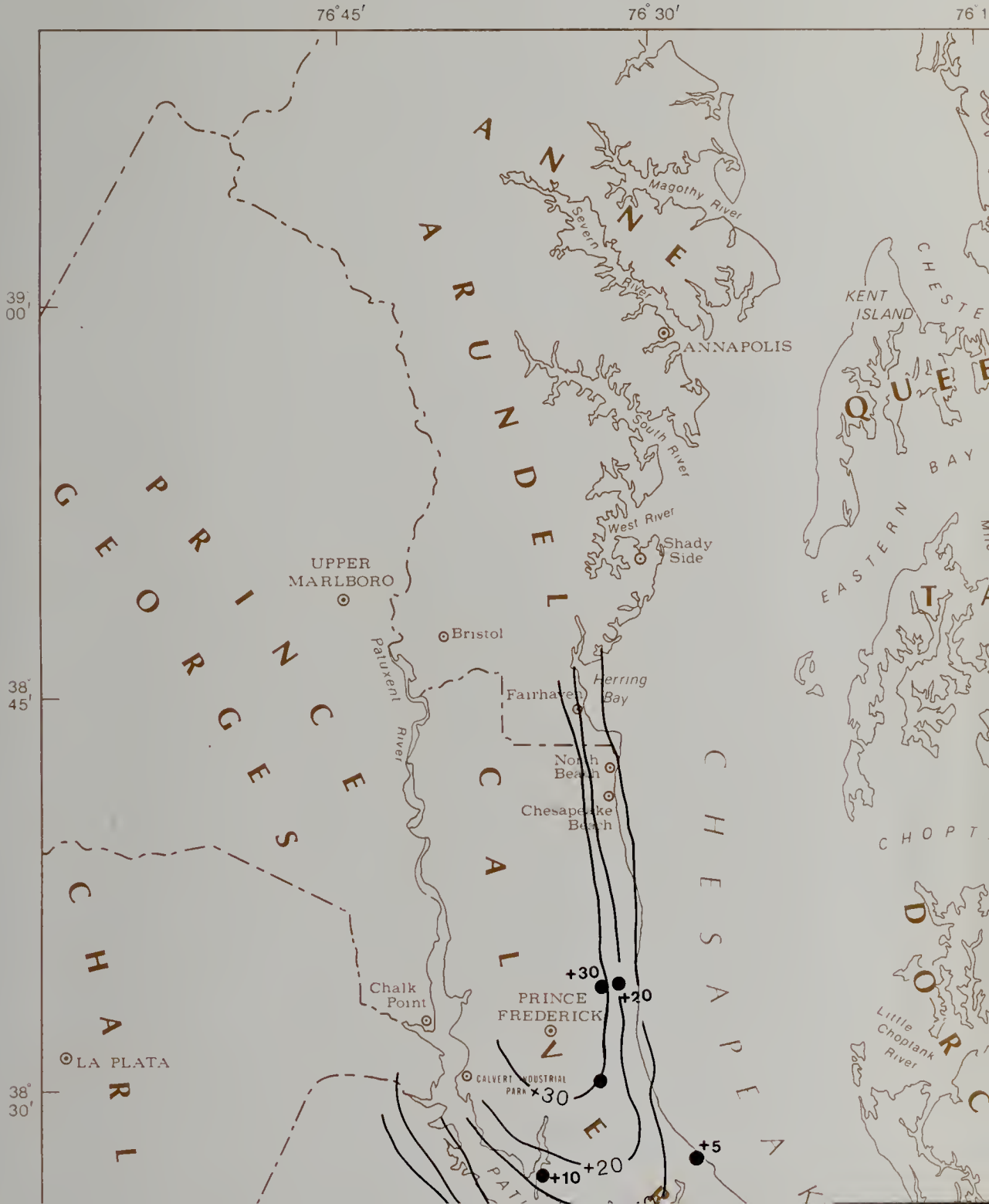
Plate 11.—Map showing simulated prepumping, 1952, and 1980 potentiometric surfaces of the Piney Point-Nanjemoy aquifer superimposed on measured water levels
