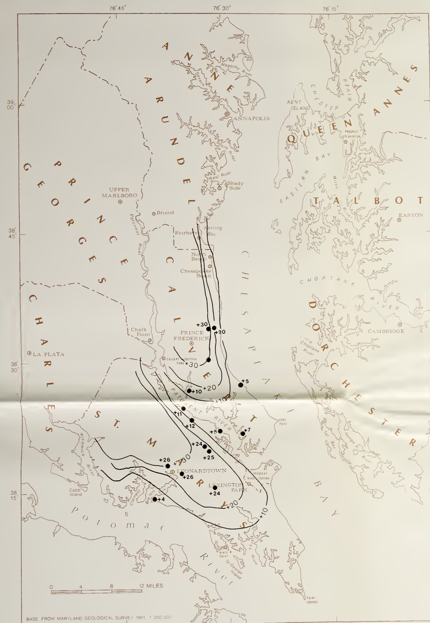
Simulated pre-pumping potentiometric surface and water levels measured early in aquifer development as reported by Darton (1896), Clark and others (1918) and Otton (1955).
