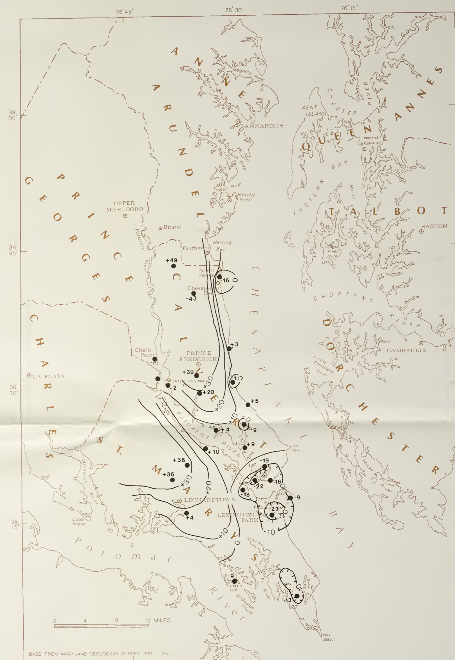
Simulated 1980 potentiometric surface and water levels measured May 19-23, 1980.
