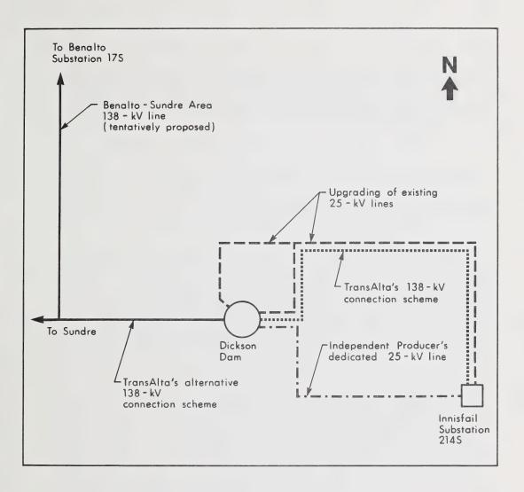
FIGURE 4: ALTERNATIVE CONNECTION SCHEMES - DICKSON DAM Applications No. 881550, 881838, 881989, 890529 Dickson Dam Power Plant
