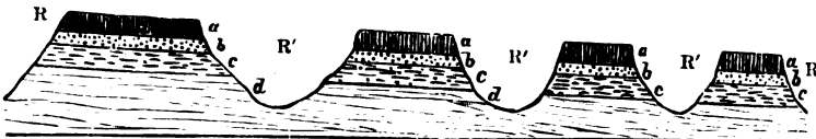
FIG. 142.—Lava-stream cut through by rivers; a, a , basalt; b, b , volcanic ashes; c, c , tertiary; d, d , cretaceous rocks; R, R , direction of the old river-bed; R', R' , sections of the present river-beds. (Le Conte from Whitney.)
