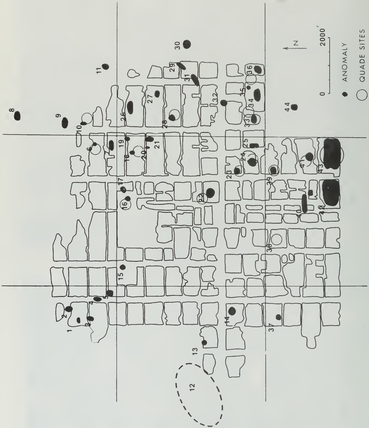
Figure 7. Anomalies and Quade subsidence sites superimposed over outlines of mine production panels.
