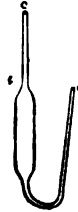
VI. — Hook-shaped Wright tube for collecting serum. Blood runs in at a until the tube is filled nearly to b . The portion bc is then warmed and the end c sealed. The air in bc on cooling draws in the blood from a . The end a may be sealed if serum is not to be used immediately.
