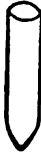
II. — Mixing tube also used for diluted sera, blood corpuscles, bacterial emulsions, etc. Made by sealing the end of a butt from mixing pipette.
