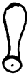
V. — Nipple for mixing the material after incubation. A thin rubber cap is cemented over a soft nipple and a hole made in its centre with a hot wire.
