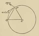
The figure represents a horizontal section of the cylinder of the screw, through the particle. O is the axis of revolution, C that of the screw, P the particle.
