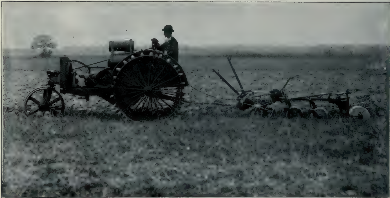
Fig. 8—An Allis-Chalmers 10-18 H.P. Farm Tractor plowing on the farm of Mr. J. S. Ainslee, near Comber, Ont.
