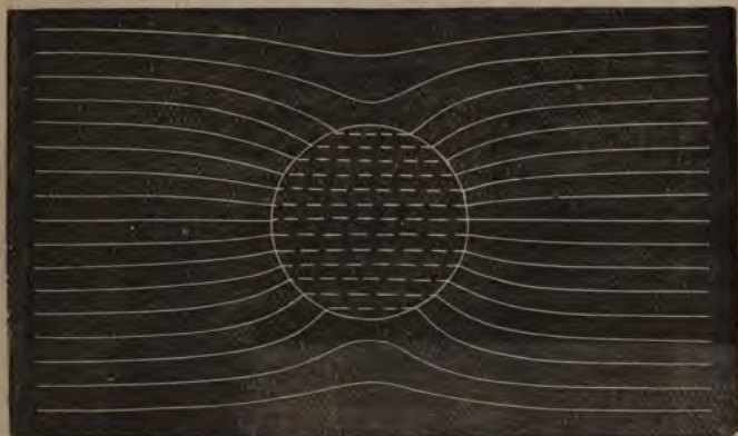
FIG. 5.—Disturbance of an originally uniform magnetic field by the introduction of a soft iron sphere.
