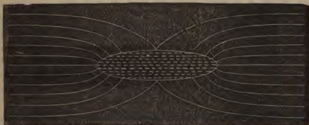
FIG. 11.—Short ellipsoid of infinitely permeable material in a uniform field.
