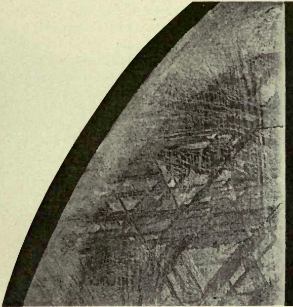
FIG. 31.—Heat crust of Charlotte meteorite. The heating of the surface in the passage of the meteorite to the earth produced the granular edge seen at the left. \times 2.5 .
