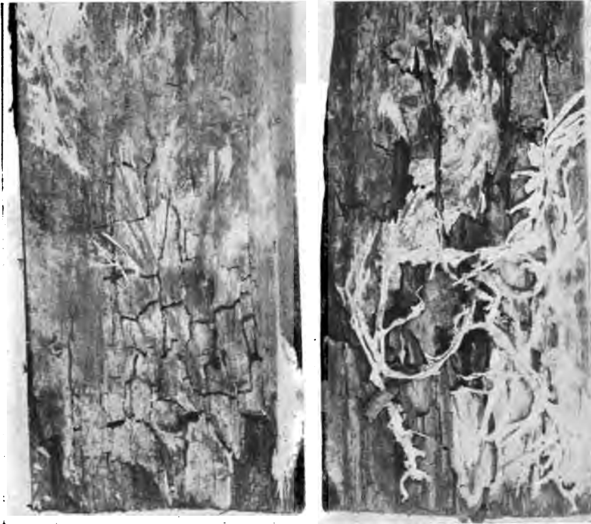
FIG. 122.—The dry-rot fungus ( Merulius lacrymans ). Later decay stages than that shown in Fig. 121. From the board shown on the left, the mycelial felt has been removed and the checked portion of the board is seen. This appearance is caused by the drawing of the tissues in drying after the decay has been well started. The removed mycelial felt is shown in Fig. 5. The board shown on the right is in a still further stage of decay and the wood under the mycelium is reduced to friable punk. Original.
