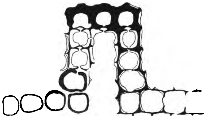
FIG. 38.—Two ways in which wood is destroyed by wood-rot fungi. On the right the wood cells are destroyed from within outwards. On the left they are destroyed from the middle of the wall toward the center of the cell. Highly magnified. After Hartig.
