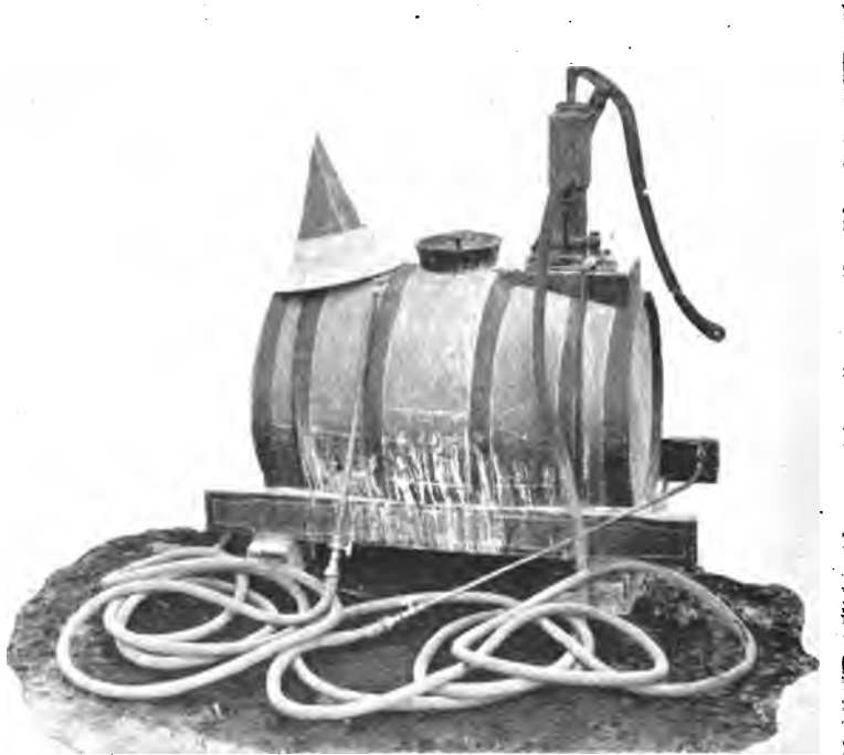
FIG. 105.—A simple type of barrel pump used in the horticultural department of the Minnesota Agricultural Experiment Station. A return pipe keeps the liquid in the barrel stirred up. The fluids are strained through the brass strainer shown above when poured into the barrel. Photograph by R. S. MacIntosh.
