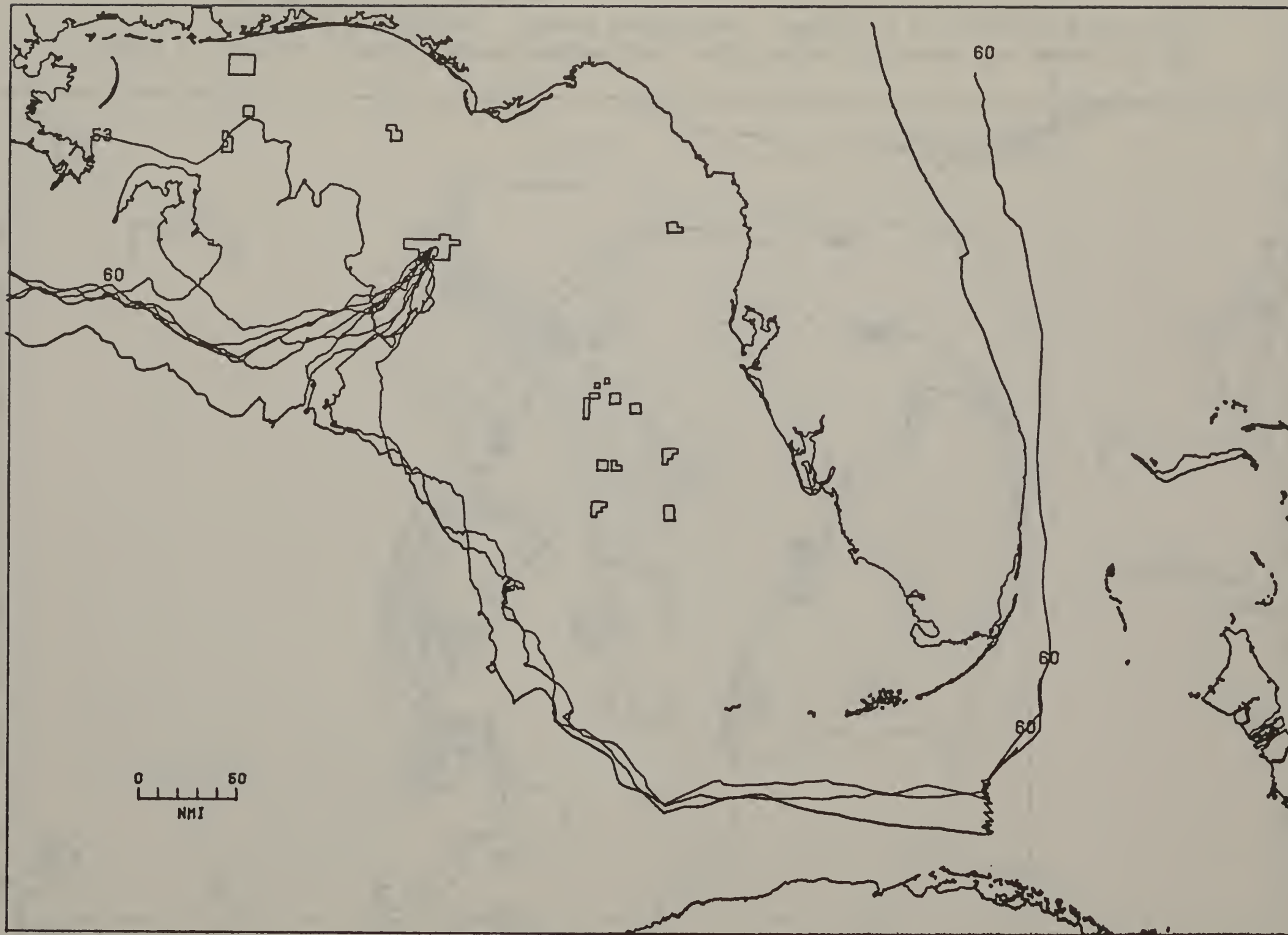
Figure 7.--Example oilspill trajectories for a spill site (P-5) near the center of the proposed lease area: autumn conditions. Number on trajectory is the time to the end point in days.
