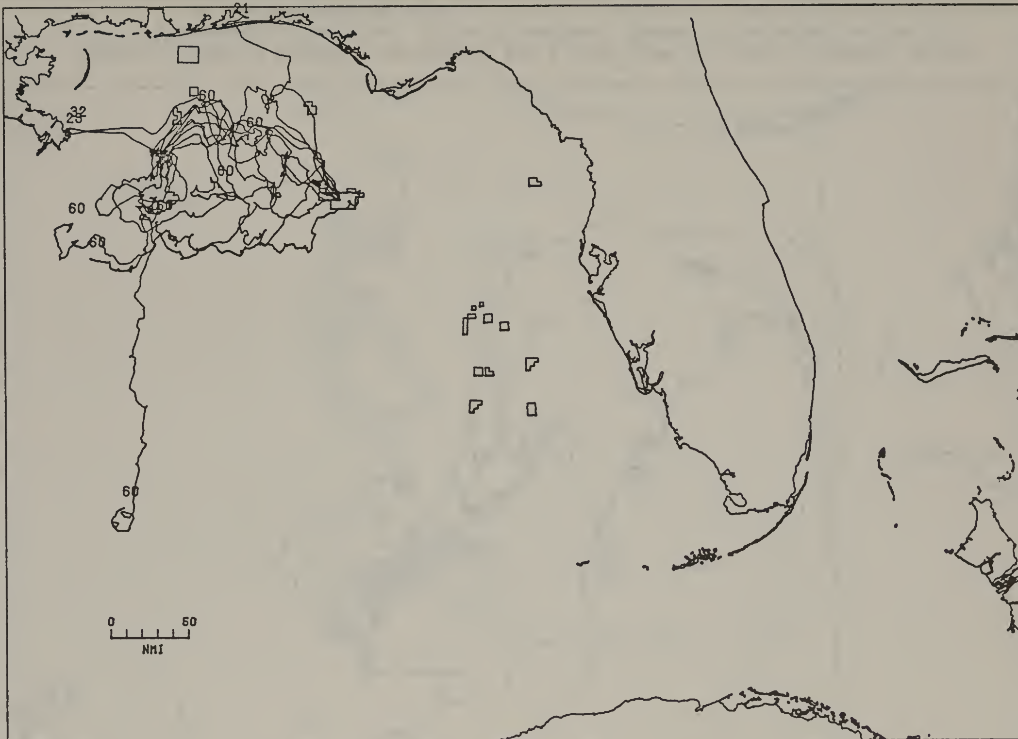
Figure 4.--Example oilspill trajectories for a spill site (P5) near the center of the proposed lease area: winter conditions. Number on trajectory is the time to the end point in days.
