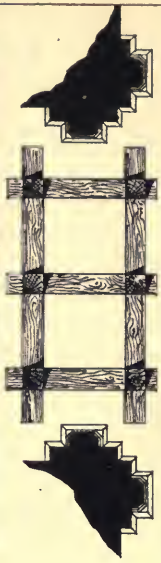
Grosmont Church; Shoring of Tower, Needling over North Arch. at Y on Plan.
