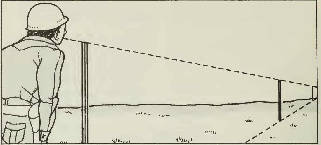
Fig. 15 Sighting a fenceline on level terrain.
